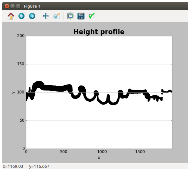
Figure D.5: Visualization of the height profile using the data extractor. The thickness of the line corresponds to the measured scatter. The height profile is updated in real time.
