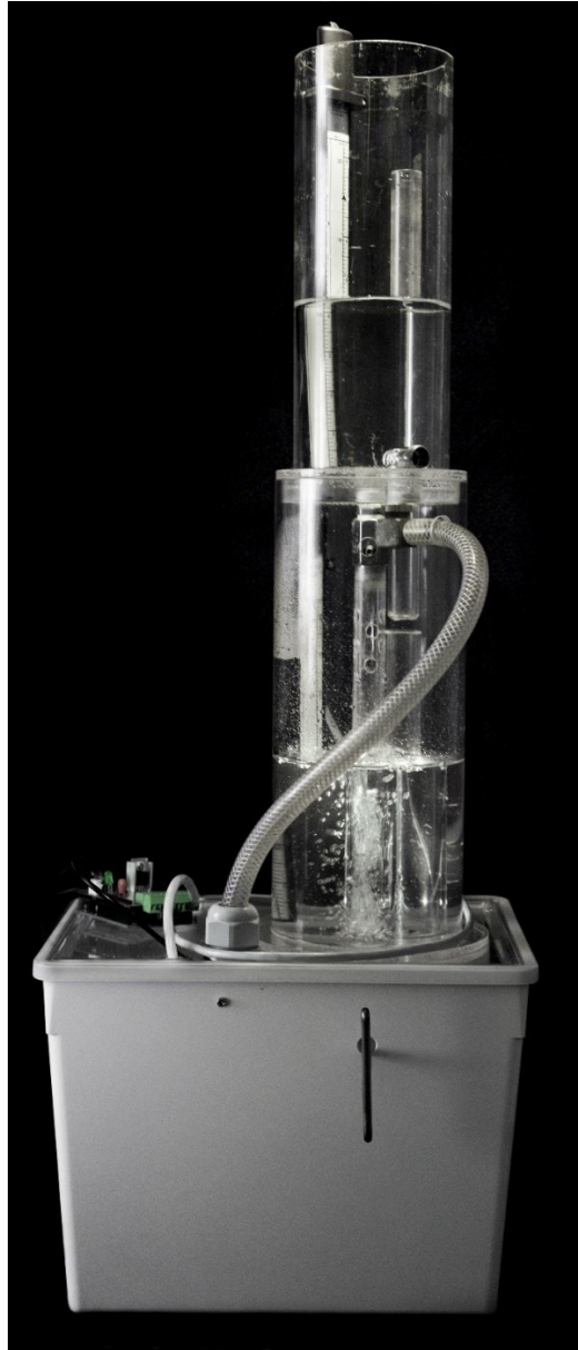
Figure 5-10: Photo of the physical STTS. Water is pumped in at the bottom of upper tank. The input flow to this tank is delivered by a submersible water pump at the bottom of the reservoir. Both tanks have a return pipe preventing overflow.
