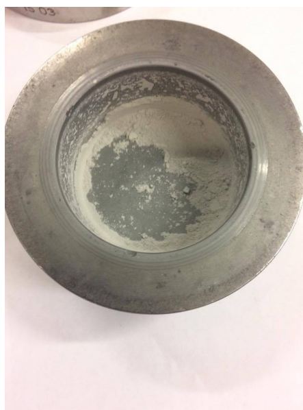
(b) Slag after crushing in ring mill
