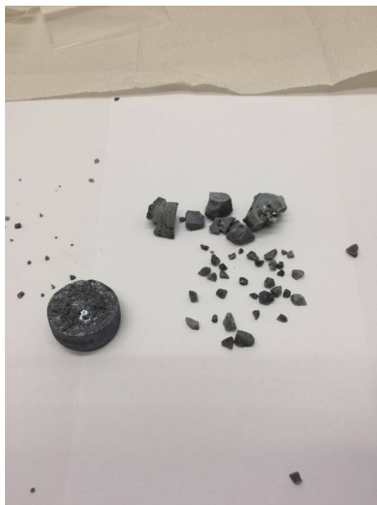
Figure 3.6: Picture of metal and slag before separation
