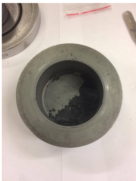
(a) Metal after crushing in ring mill
