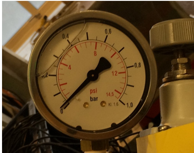
Figure 4.3: The output pressure from the compressor during the experiment.
