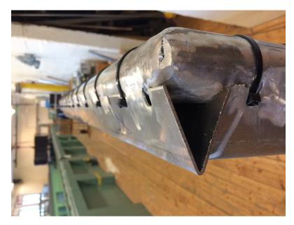
Figure 3.2: Strips layout. The net was stretched by the plastic strips and the strips went through the holes on the frame and were tied at the outer side of the frame.
