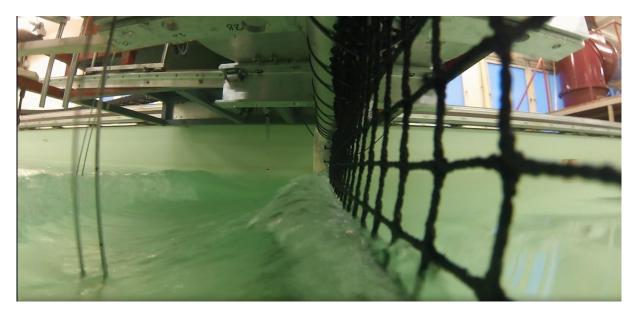
Figure 4.2: Screenshot from the video about the surface elevation behind the net during towing process.
