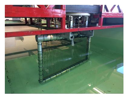
Figure 3.1: Experimental set-up. The red steel frame is part of the carriage system. The silver steel frame was fixed onto the carriage at the top middle side, with two sensors installed measuring the forces. Six wave gauges were fixed at different locations in front of or behind the net to measure the surface elevation.
