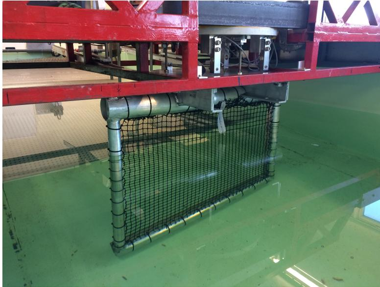
Figure 3.1: Experimental set-up. The red steel frame is part of the carriage system. The silver steel frame was fixed onto the carriage at the top middle side, with two sensors installed measuring the forces. Six wave gauges were fixed at different locations in front of or behind the net to measure the surface elevation.
