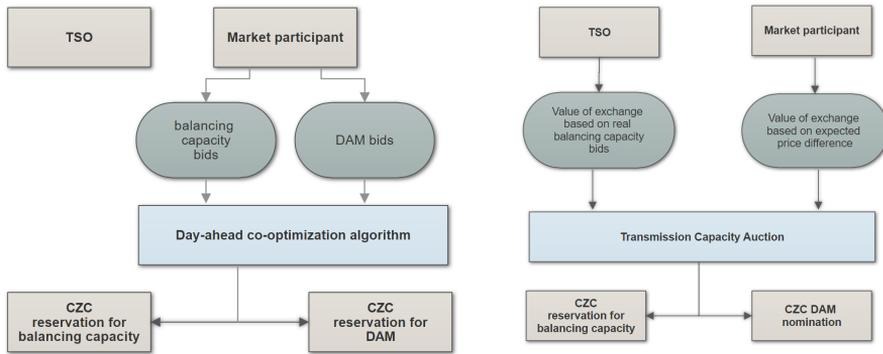
**Figure 4.3:** Flow chart of a co-optimization model with an implicit(left) and explicit(right) auction. The figure is based on [29].
