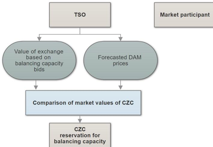
**Figure 4.4:** Flow chart of a market-based reservation model. The figure is based on [29].
