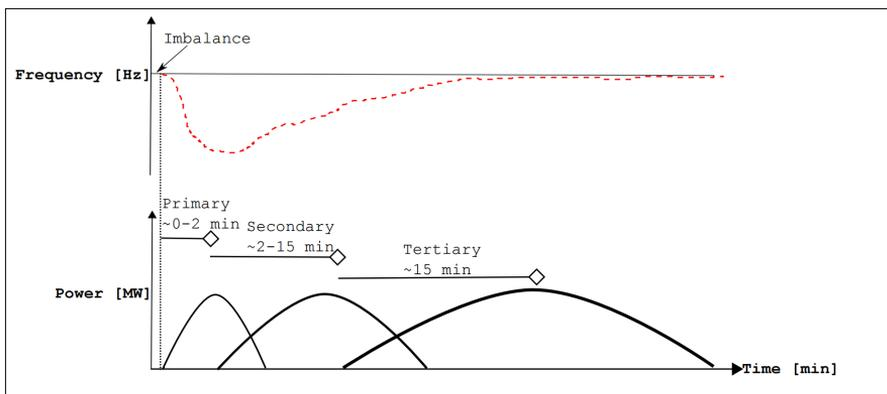
**Figure 2.2:** Balancing services. Figure collected from [14].
