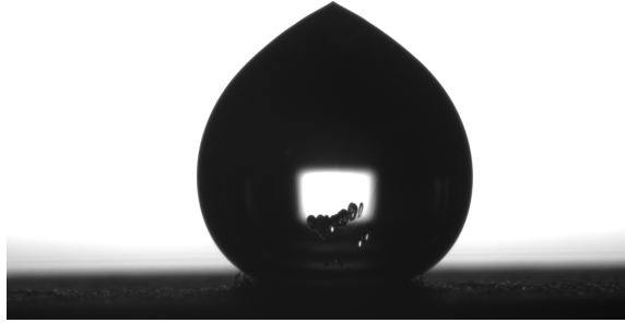
Figure 4.23: A picture showing a droplet frozen through the second freezing mechanism.
