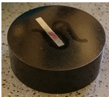
Figure 4.10: A picture of sample C-S1-L2 that has been molded into thermoplastic, then ground and polished to expose its cross section.
