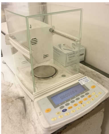
Figure 3.6: The Sartorius ME235P analytical balance scale used for weight measurements.
