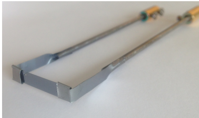
Figure 4.6: Silicon evaporator . A piece of silicon wafer is connected to the chamber in such a way that a current can flow through it. The temperature increases until silicon evaporates, covering the sample substrate.
