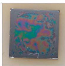
Figure 8.4. Example of spin-coated film (Ti-PDMS-65-2:1).
