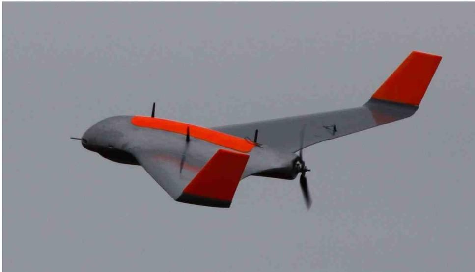
Figure 3.3: Skywalker X8 Flying Wing airframe. Photo: NTNU Unmanned Aerial Vehicles Laboratory (UAV-Lab).
