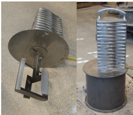
Figure 3.5: ConTec Rheometer-4SCC apparatus. Extracted from [55].
