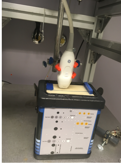
Figure 3.6: Experiment setup showing the probe, how the probe is attached to the stepper motor and the phantom. The phantom is filled with water on top.
