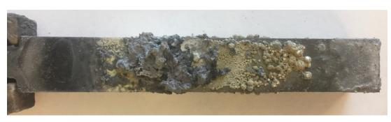
Figure 6.1: Composite sample 3018g after completed wetting test.
