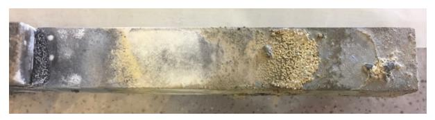
Figure 6.3: Composite sample 3112g after completed wetting test.
