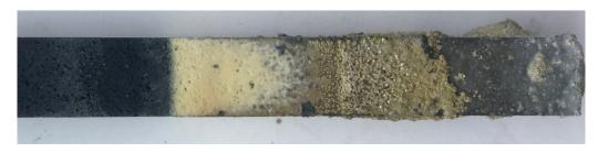
Figure 6.9: Composite sample 6004g after completed wetting test.
