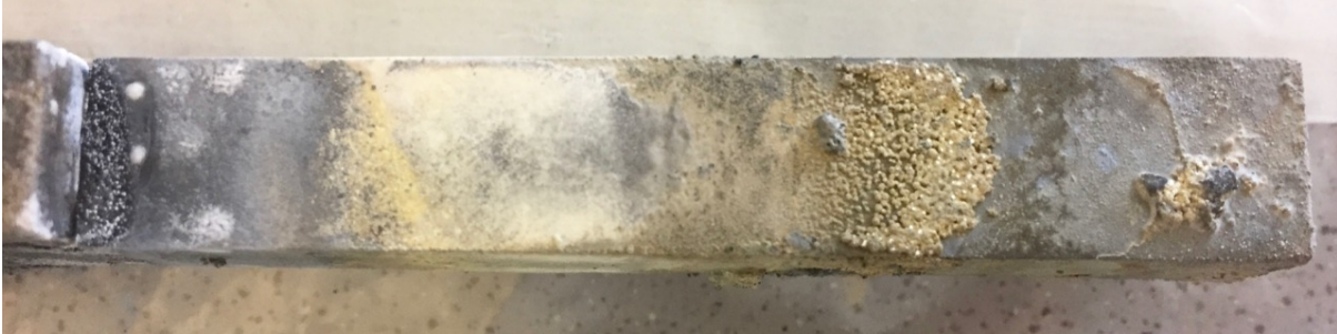
Figure 6.3: Composite sample 3112g after completed wetting test.
