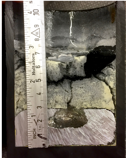
Figure 4.5: Cross-section of crucible with solidified electrolyte and metal after completed wetting test.
