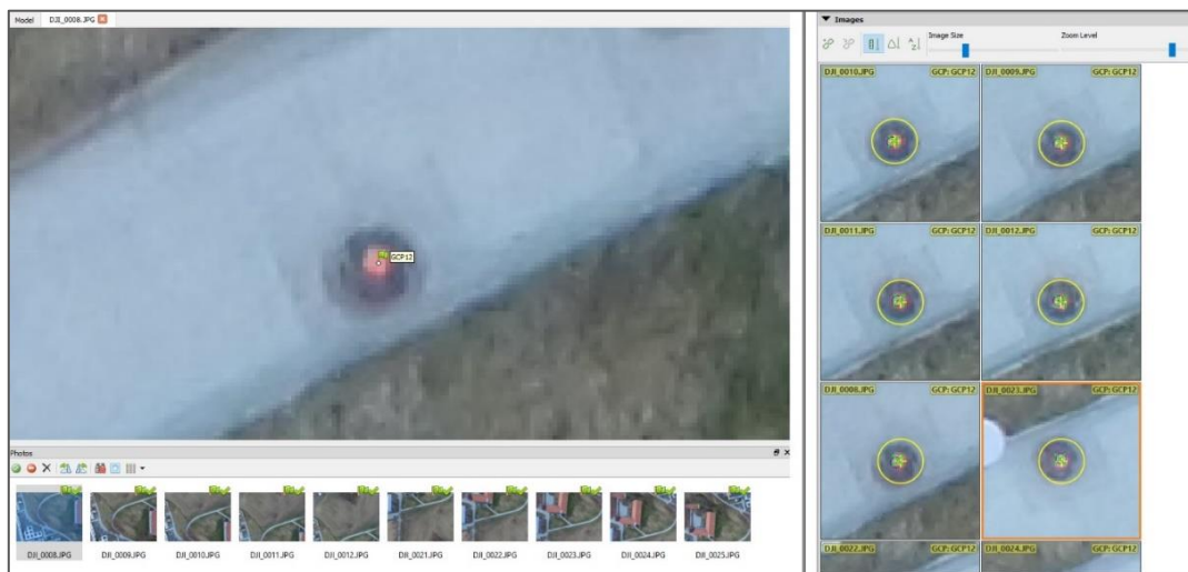
Figure 12 Manual measurements of control points in Agisoft (on the left) and in Pix4D (on the right)
