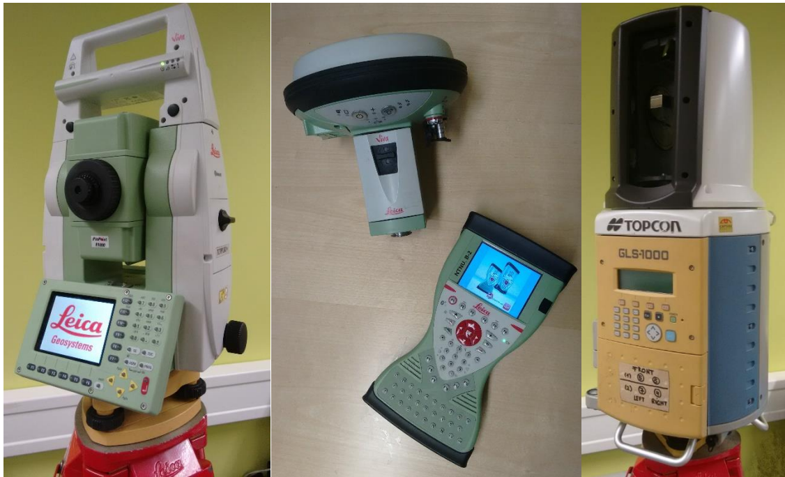
Figure 23 Total station (left), GNSS receiver (middle) and laser scanner (right) used in measurements.
