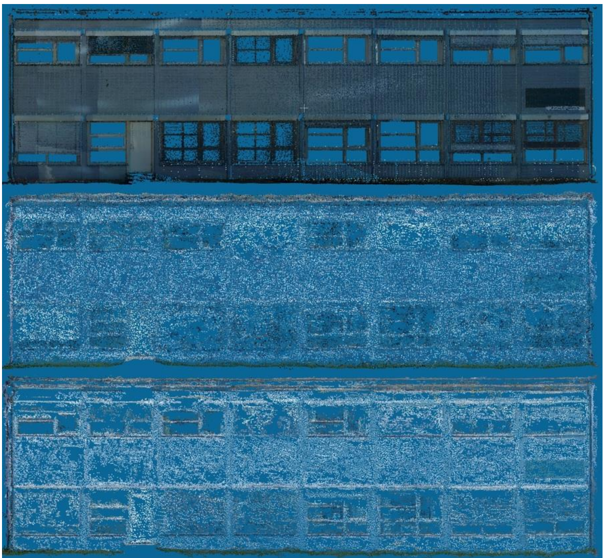
Figure 37 A wall represented by point cloud obtained from laser scanning (upper), Agisoft PhotoScan (middle) and Pix4D (lower).
