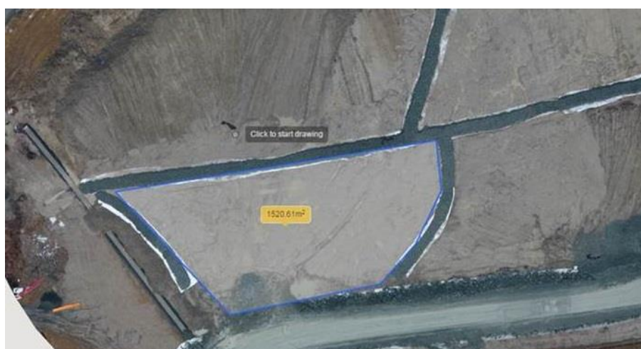
Figure 7 Surface measurements. Source: Statens Vegvesen.
