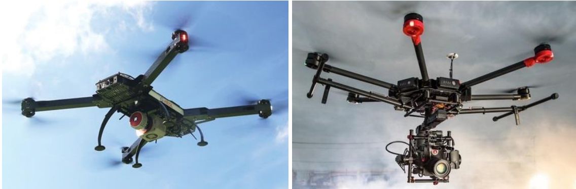
Figure 11 UAV with mounted laser scanner (on the left), source: www.insideunmannedsystems.com , and professional camera (on the right), source: www.macnn.com .
