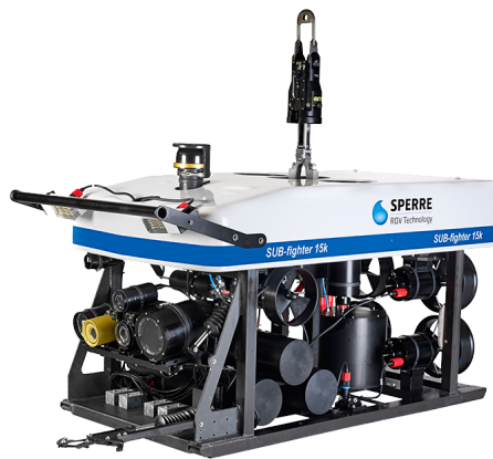
Figure 2.4: A typical ROV used for aquaculture operations (Sperre, 2016).
