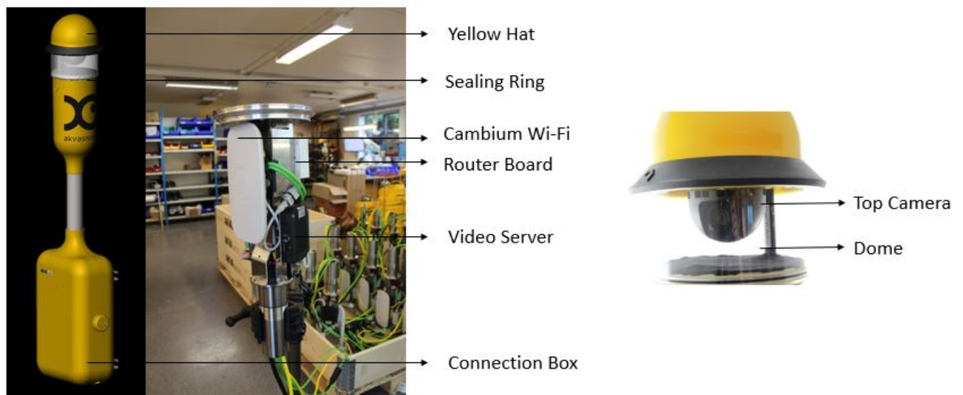
Figure 6.7: Cage Access Point by AKVA Group 15,16
