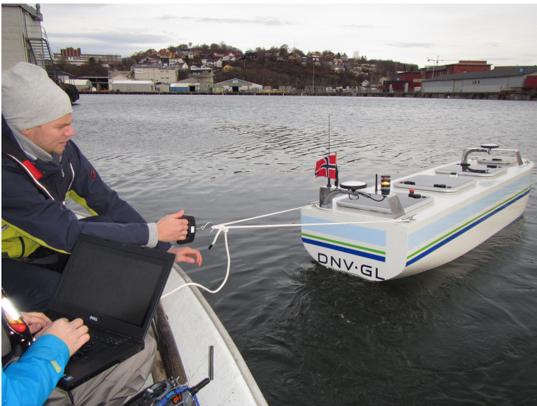
Figure 8.6: Kjetil performing a bollard pull test with a luggage scale. Photo by Egil Eide.
