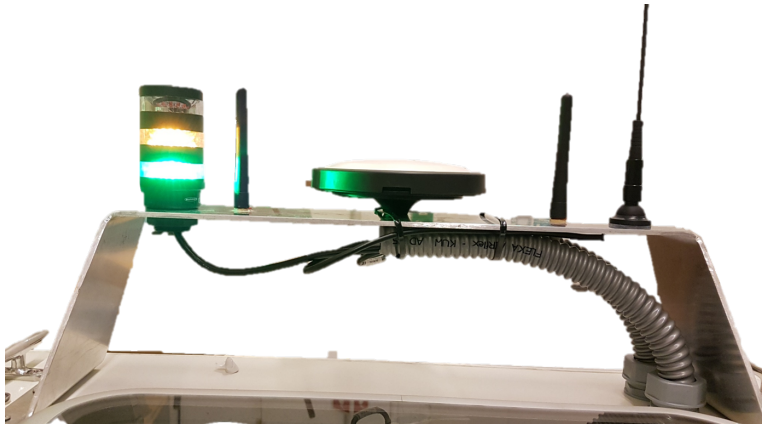
Figure 6.7: Close up of the stern boat tower. From the left: Light beacon, Wi-Fi antenna, GNSS antenna, Wi-Fi antenna, radio link antenna.
