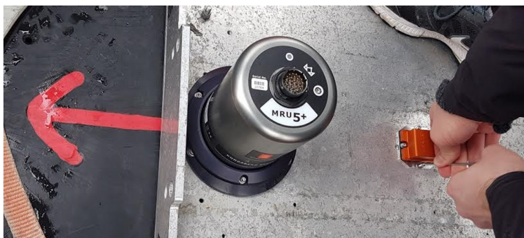
Figure 10.1: Mounting of Seapath and Xsens IMUs on Telemetron.
