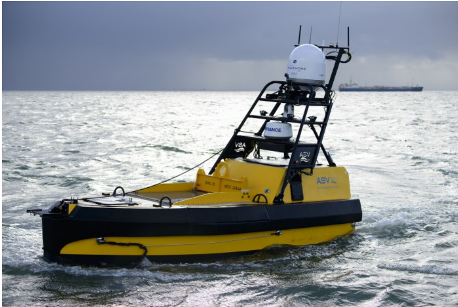
Figure 1.1: The C-Worker is a multiuse offshore ASV developed to conduct subsea positioning, surveying and environmental monitoring for oil and gas operations. Courtesy of [1].
