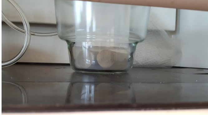
Figure B.3: SurfaSil saturation of core sample T1 and T2
