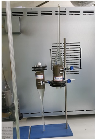
Figure 5.2: Amott experiment on cores T1 and T2
