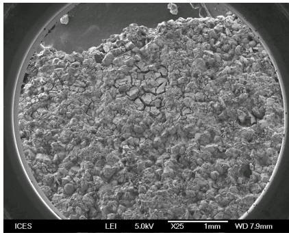
(a) SEM-image of sand grains at x25 magnitude
