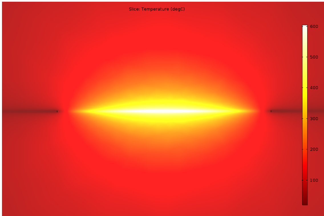
Figure 6.1: Heat distribution over wolfram wire with a diameter of 0.38 mm, simulated in COMSOL.
