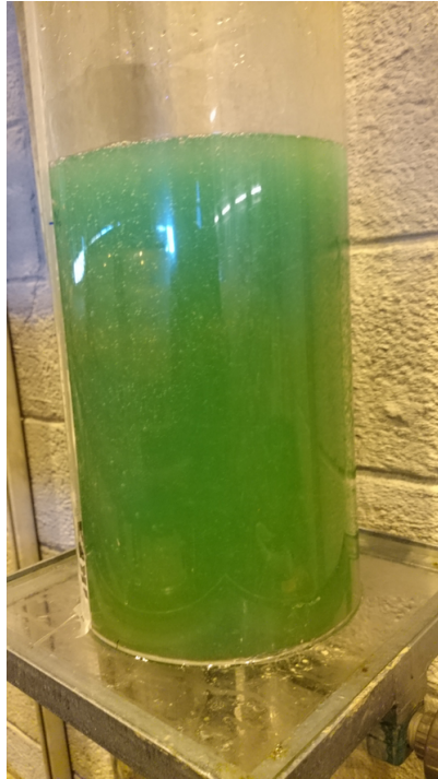
Figure 5.3: The collector tank with the two fluids before they were thoroughly mixed and conductivity measurements were performed.
