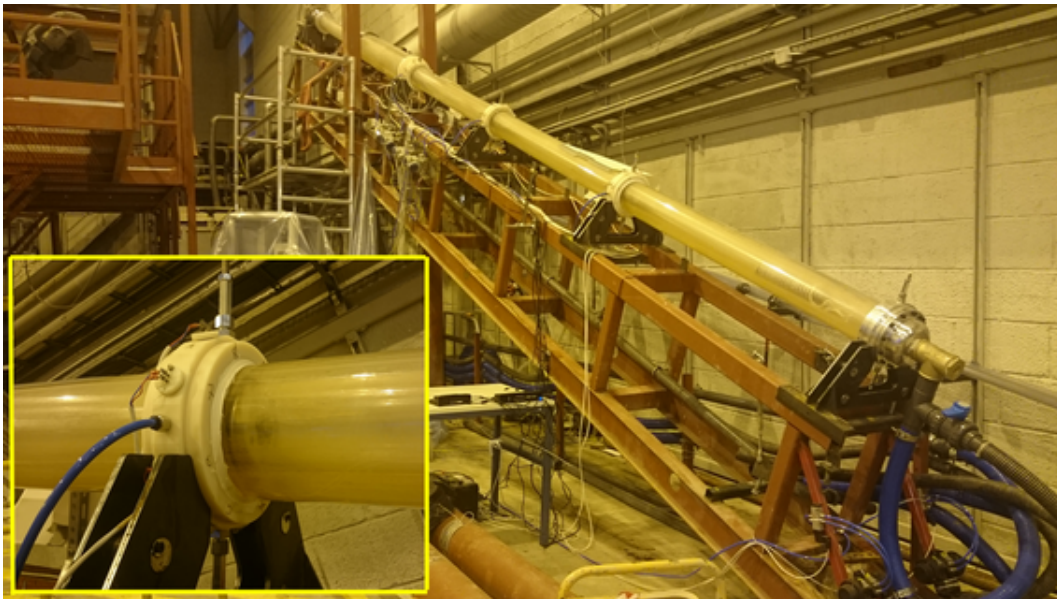
Figure 4.9: Large scale flow loop. Small picture shows a sampling point for pressure and salinity, together with the adjusting mechanism for the eccentricity (Giil and Johansen, 2016).
