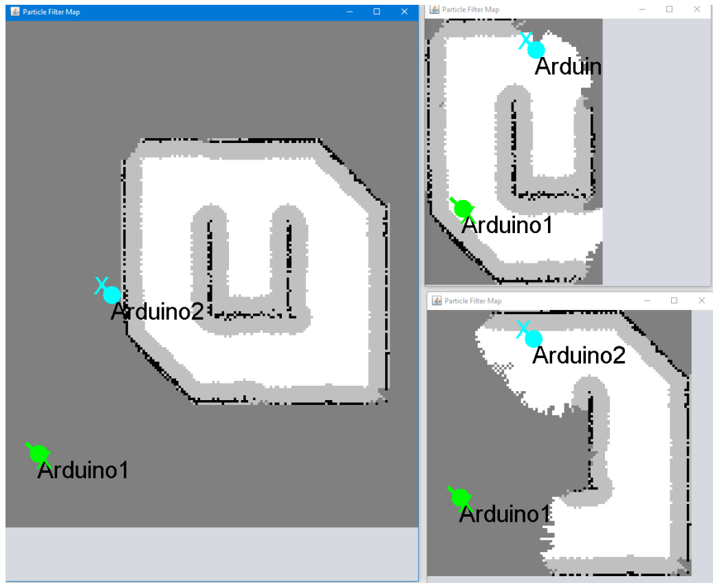
Figure 3.2: This figure shows how the two partially overlapping maps can be combined using the map merging algorithm. The c_{lock} value was set to 100.
