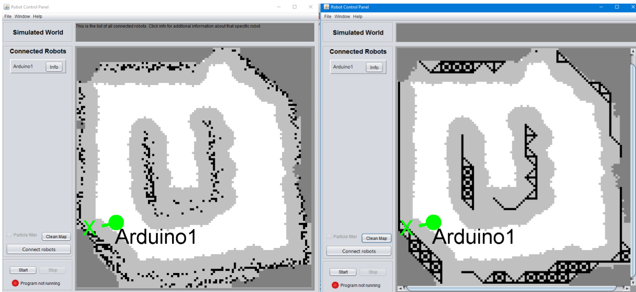
Figure 6.2: The CleanMap algorithm on a poor map. Left is before, and right is after the CleanMap function is run
