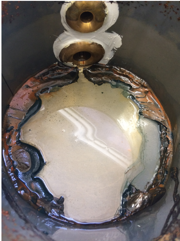
Pictures above: After 24 hours of circulation the container had corroded and particles had accumulated at the bottom.
