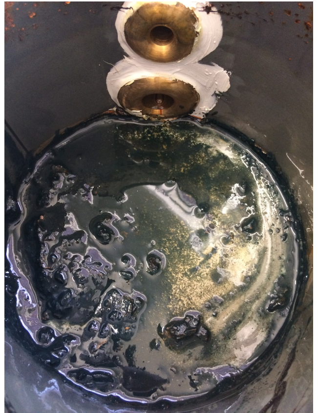
Pictures above: After 24 hours of circulation the container had corroded and particles had accumulated at the bottom.
