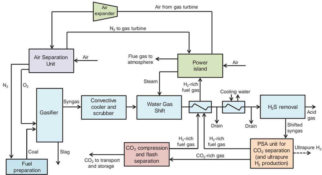
Figure 1. Flowsheet of a general IGCC plant with CO<sub>2</sub> separation and coproduction of H<sub>2</sub> by PSA.
