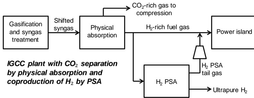
Figure 4. Block-flow diagram of the IGCC plant with CO<sub>2</sub> separation by physical absorption and coproduction of H<sub>2</sub> by PSA.
