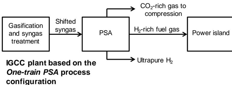
Figure 3. Block-flow diagram of the IGCC plant based on the One-train PSA process configuration.
