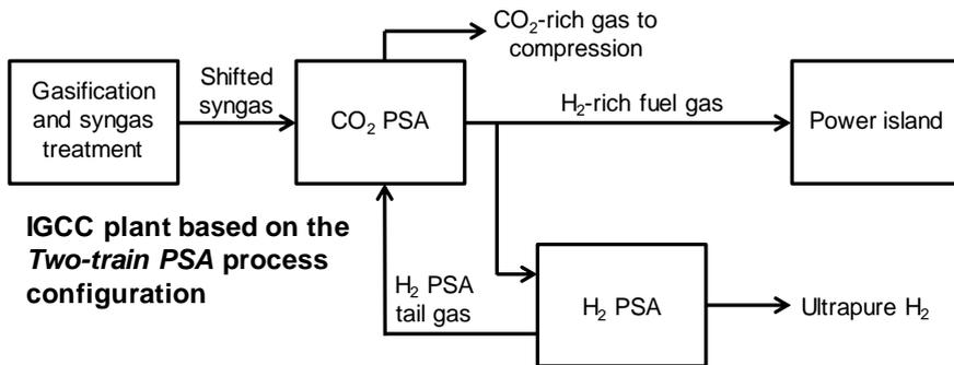
Figure 2. Block-flow diagram of the IGCC plant based on the Two-train PSA process configuration
