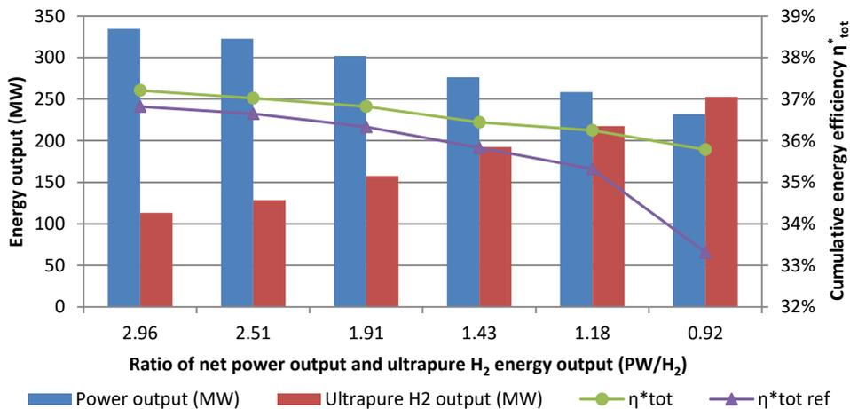
Figure 5. Share of energy products at different plant loads. The different cases are named after the ratio of net power output and ultrapure H<sub>2</sub> energy output (PW/H<sub>2</sub>). The performance of the Two-train PSA process configuration is also reported in terms of cumulative efficiency (η\* tot), together with the performance of a reference IGCC plant for power generation implementing CO<sub>2</sub> capture through absorption and without any H<sub>2</sub> production (η\* tot ref).
