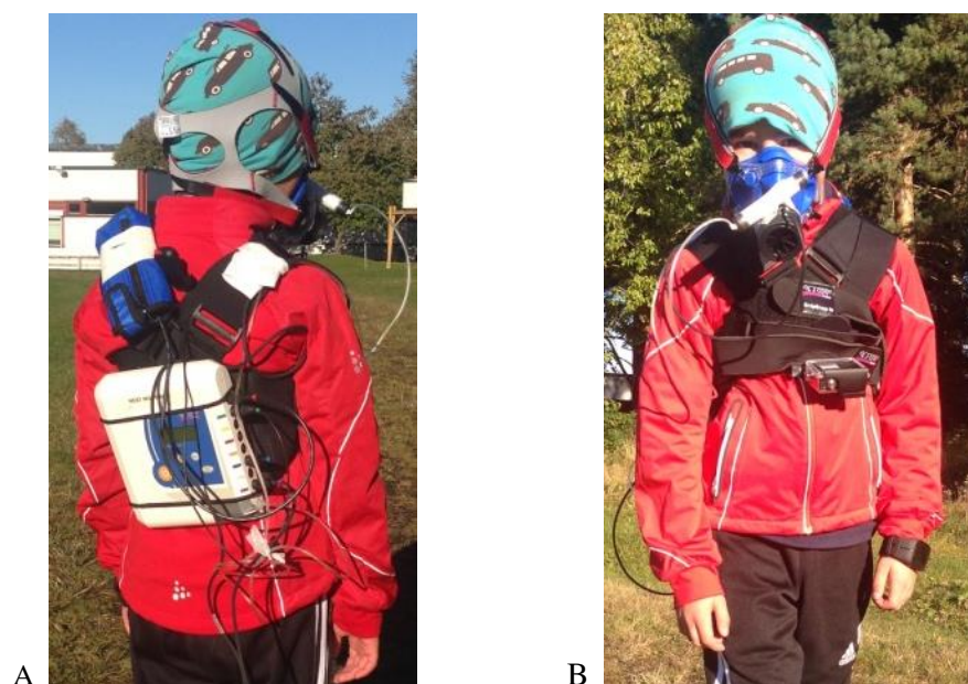
Figure 1 Equipment setup with Metamax (A) and facemask (B).
