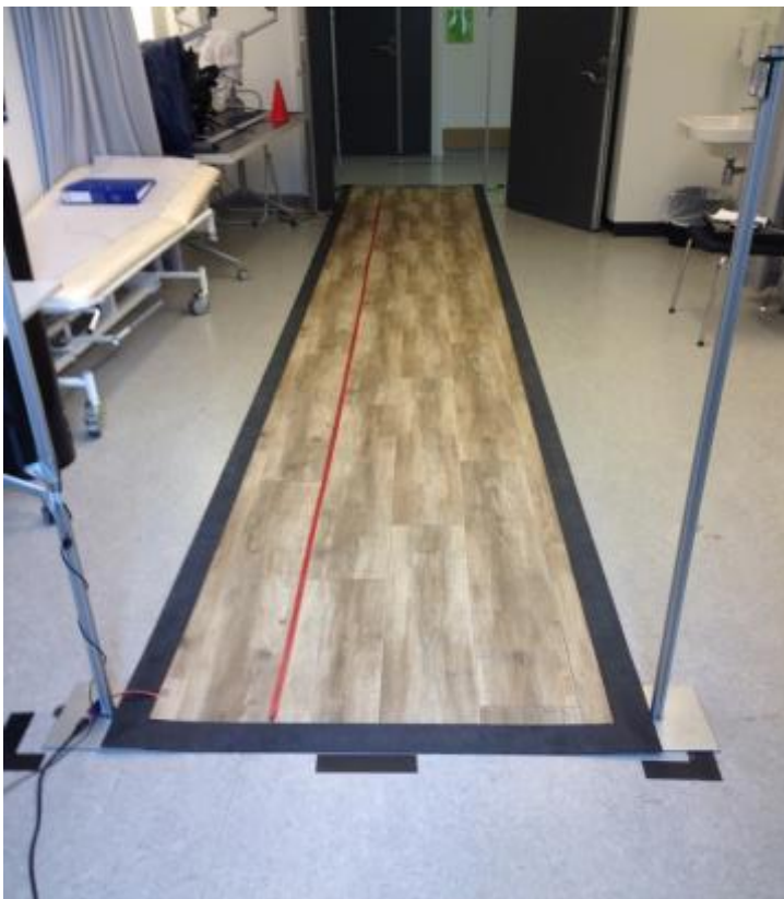
Figure 1: This is the Zeno walkway that participants walked on, with the red marking where the active sensors are (to the right of the red line).
