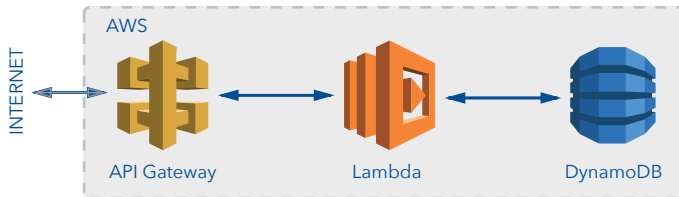
Figure 4.1: Relation between AWS components to achieve a server-less application architecture.
