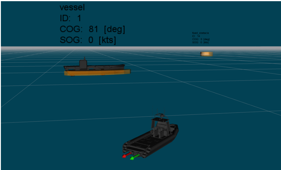
Figure 7.4: Odin during simulation of the busy open sea scenario. Detected objects broadcast by the simulated TDM are illustrated as partially transparent, orange discs, representing the estimated size, position and heading of the object. A descriptive keyword, the object's given ID, COG and SOG are illustrated as text hovering above the estimated position of the detected object. Arrows representing the angle and force of thrust are connected to Odin's thrusters.
