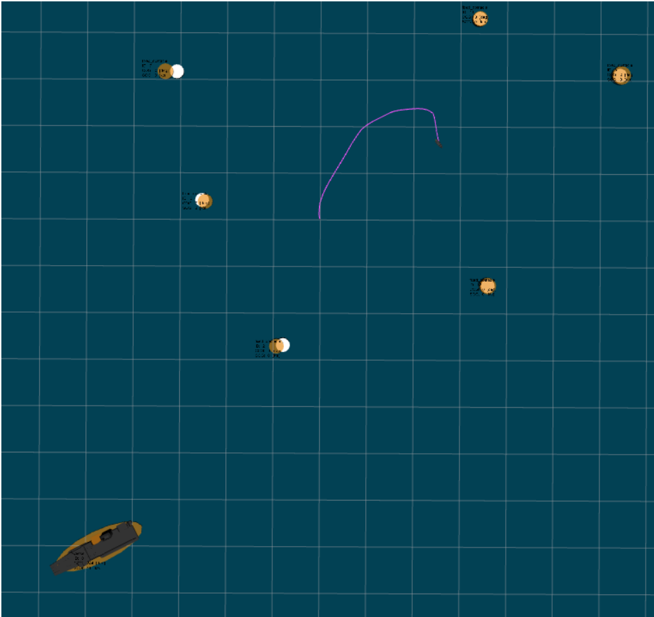
Figure 7.5: The busy open sea scenario seen from above, illustrated in RViz. The path of Odin is visible as a purple line.
