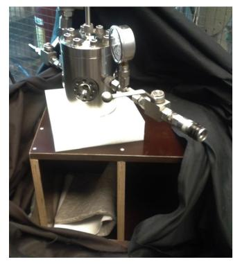
Figure 28. Insulating and stabilizing designed base for the pressure vessel to locate that one at the desired height.
