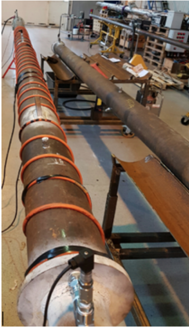
(a) Instrumenting cells with heating cables.
