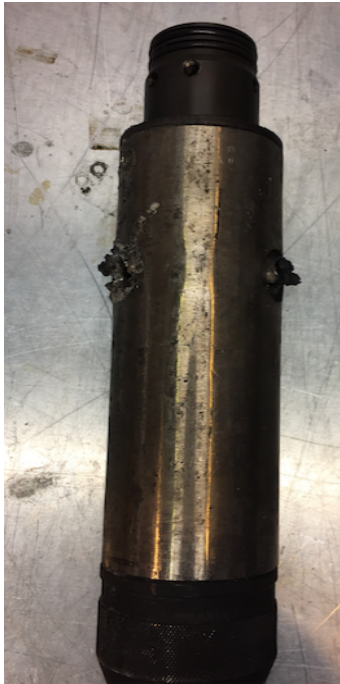
Figure F2: Photo of perforation module after firing (3 shots)
