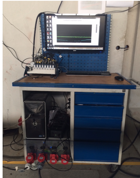
(b) Panel used for monitoring and controlling pressure and temperature data.
