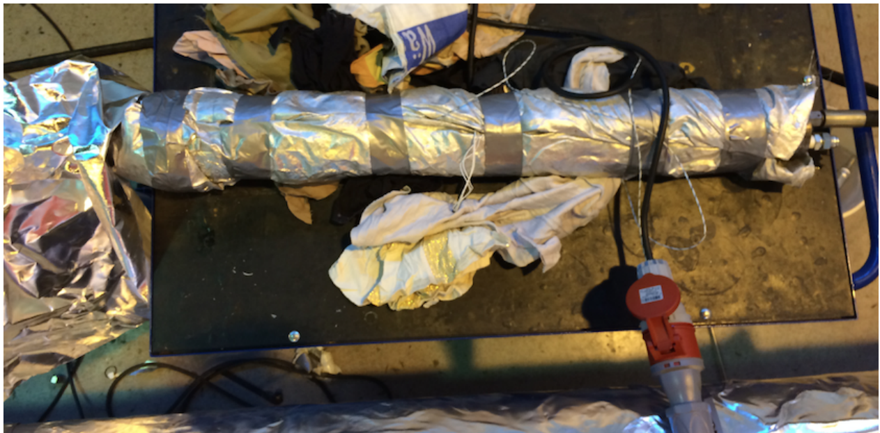
Figure F3: Photo of sample-cell used for storing and pumping of resin for cells one and three. The sample-cell is installed with heating cables.
