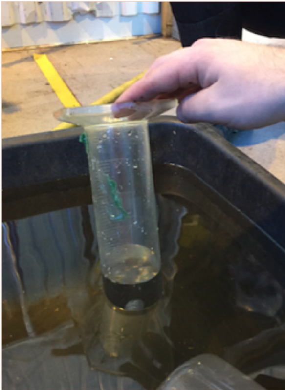
(a) Gas leaking measurement.
