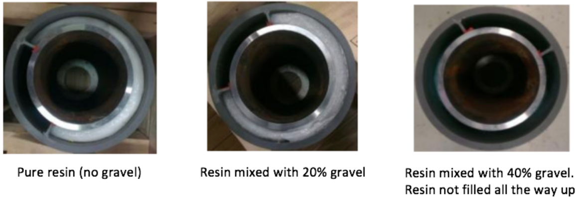
Figure 2.16: Showing the three different annular filled with different resin systems. Courtesy of Schlumberger.
