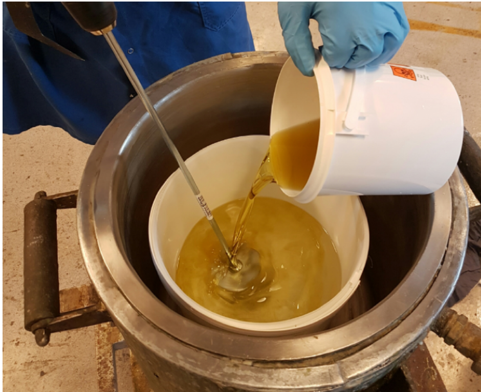
Figure 3.11: Mixing of the resin. Picture shows the addition of hardener system.
