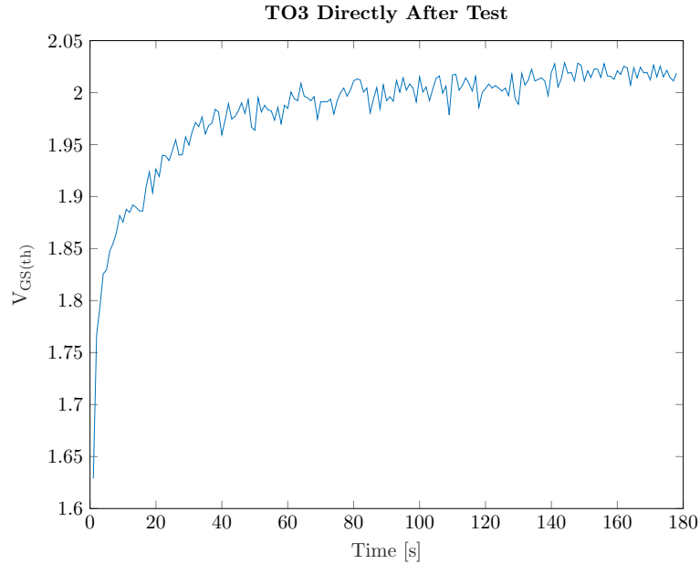
Figure 3.6: Threshold voltage of TO3 directly after test
