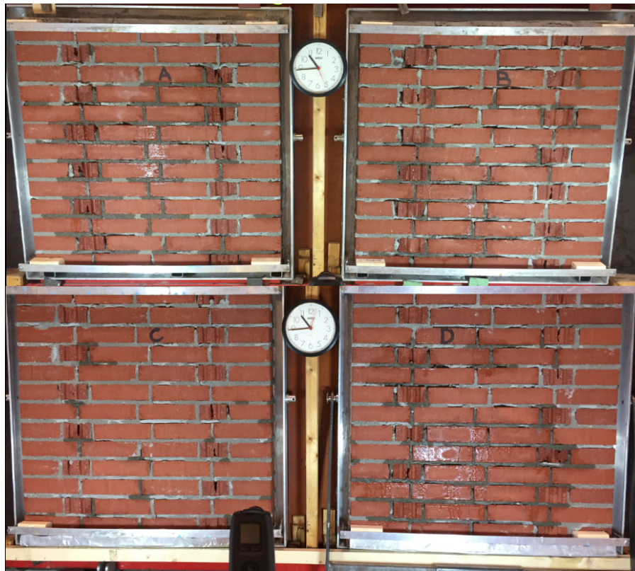
Figure 4. Panels A, B, C, and D after 45 min of simulated driving rain.
