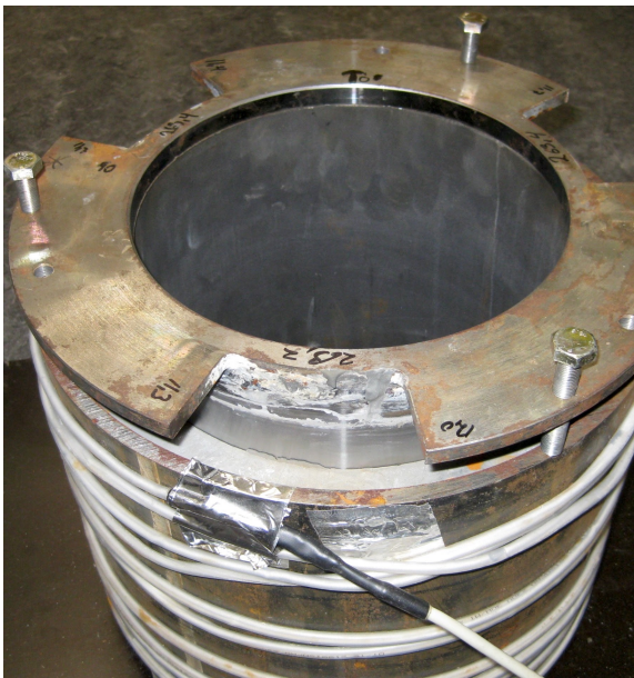
Figure 4.13: Microannulus generation by hoisting the tapered casing.
