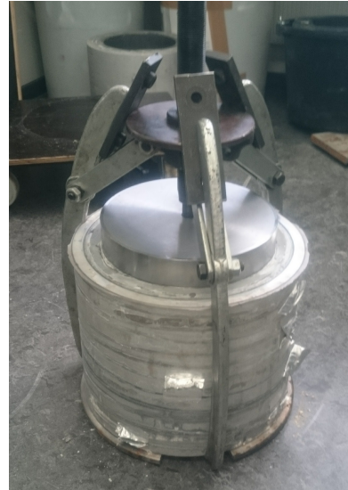
Figure 4.5: Using hydraulic puller to break casing-cement bond (note that the sample is upside down).
