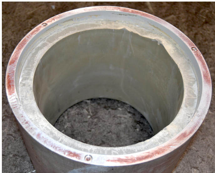
Figure 4.10: Inspection of the cement sheath quality after pulling the casing from a sample using coated aluminum.
