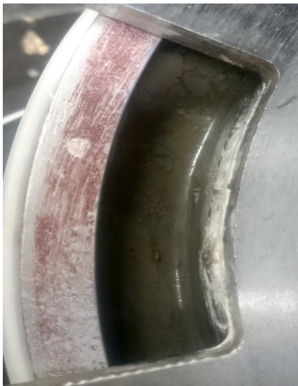
Figure 4.9: Sample with coated aluminum during initial hydration. No generation of gas was observed.
