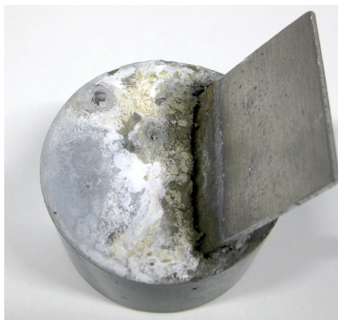
Figure 4.11: Test of aluminum corrosion in cement without steel present – for evaluating the possibility of coating steel casing.
