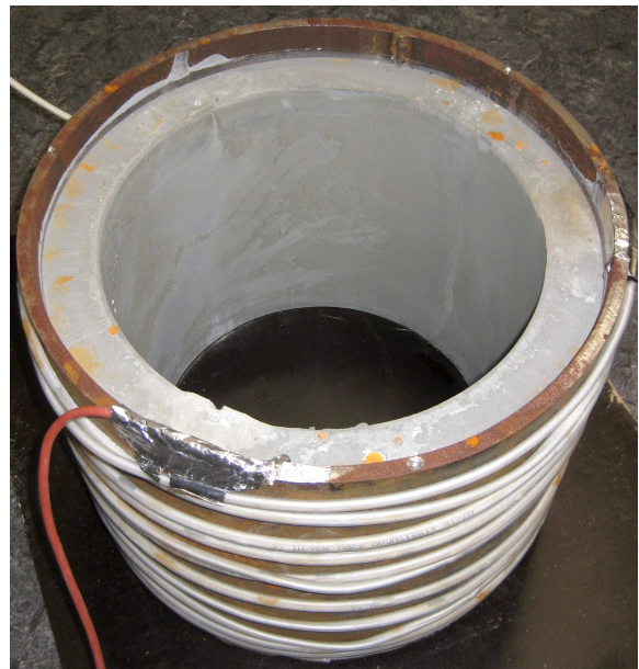
Figure 4.14: Visual inspection of the cement sheath quality by pulling the casing after logging.
