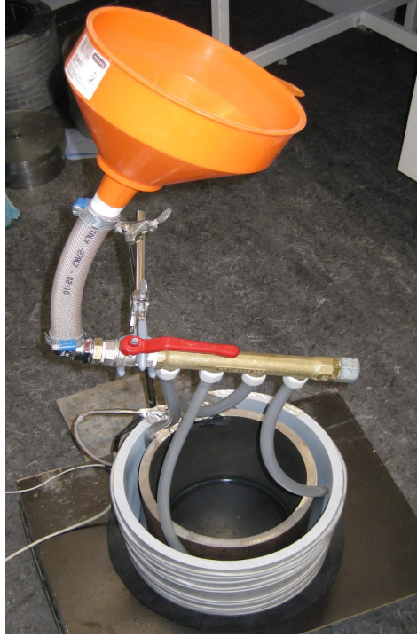
Figure 4.1: Equipment rigged up for cementing of the annulus.
