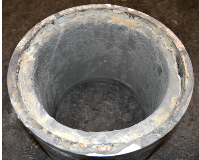
Figure 4.7: Inspection of the cement sheath quality after pulling the tapered casing.
