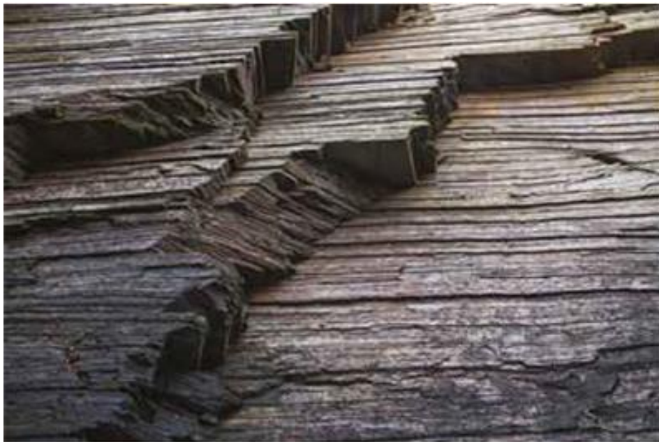
Figure 2-1 Example of a shale formations laminate structure according Norton (2016)
