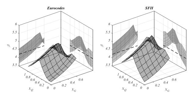
Figure 2. Reliability indices for Case 1, compression parallel to grain  $F_{c,0}$ , dominating variable loads and solid timber: Eurocodes (left), calibrated SFII (right) and Eurocodes weighted average (dashed line).
