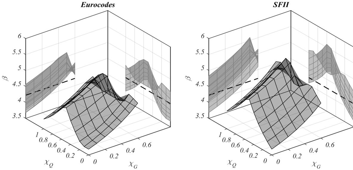
Figure 2. Reliability indices for Case 1, compression parallel to grain  $F_{c,0}$ , dominating variable loads and solid timber: Eurocodes (left), calibrated SFII (right) and Eurocodes weighted average (dashed line).
