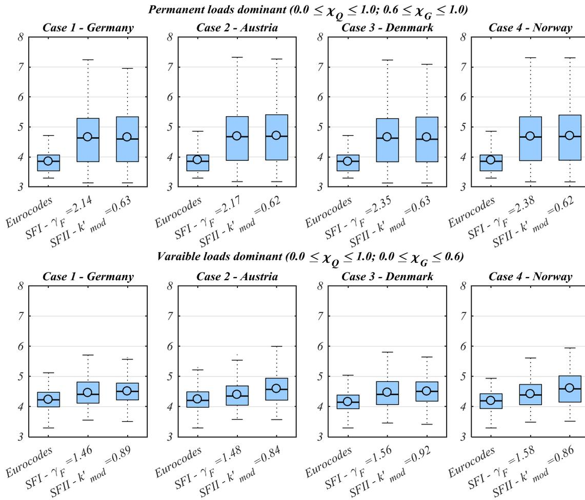
Figure 1. Reliability indices corresponding to the design performed with Eurocodes and the two simplified safety formats with calibrated reliability elements for ST dominating (Box-and-whisker plot with boxes from first to third quartiles with median (line) and mean value (circle), whiskers from minimum to maximum).
