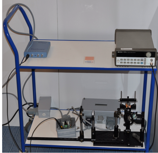
Figure 3.8: An image of the prototype setup placed on a rolling table. In the image the following components are visible, starting from the top left: the Picoscope oscilloscope, an IR-sensor card, a signal generator, power supply for Laser Gas 2, the detector board, in front the optical setup shown in figure 3.9, and in the back the main unit of NEO's Laser Gas 2.
