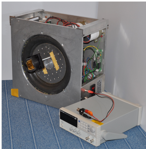
Figure 3.7: An image showing the retroreflector mounted on the 12" subwoofer(speaker), for oscillating the object. The subwoofer was driven with a 0.5 Hz triangular modulation, which resulted in a peak-peak movement of approximately 1 cm, which results in a velocity of 0.01 m/s.
