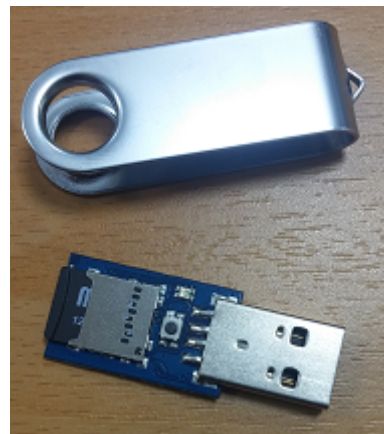
Figure 11: Picture of the inside of the USB Rubber Ducky
