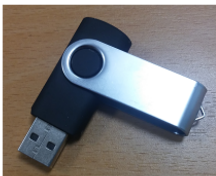
Figure 10: Picture of the USB Rubber Ducky when completely assembled
