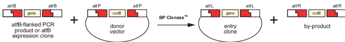
Figure 2.1 A recombination reaction aided by BP Clonase™ II, ensures that desired PCR product flanked by attB sites is inserted into appropriate donor vector with attP sites. An entry vector and a by-product is the result of correct recombination (Invitrogen, 2004).
