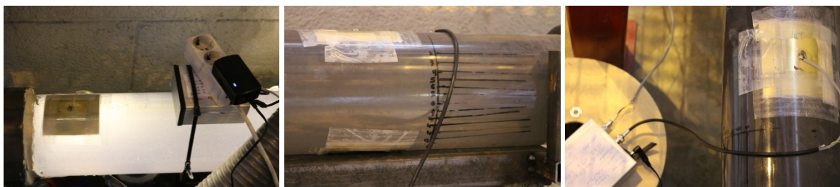
Figure 4.9: Electrodes placed at the pipe wall
