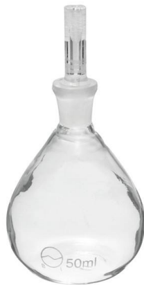
Figure 4.17: Pycnometer for density measurements
