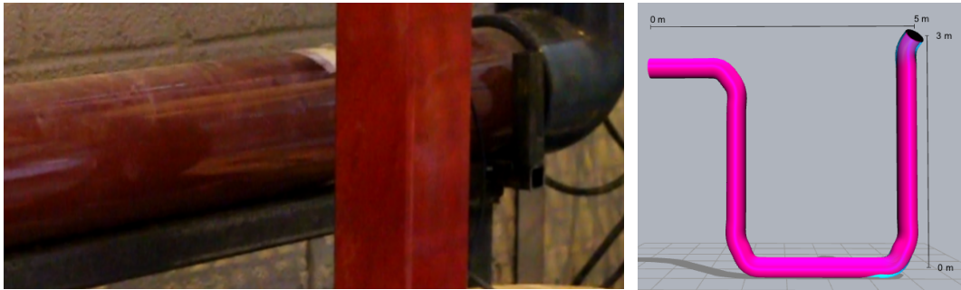
Figure F.3: Pictures of experiment and LedaFlow model at different times, for oil displacing water at 28.164 m 3 /h
