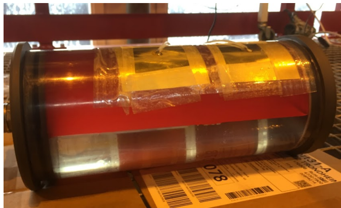
Figure 4.11: Calibration cylinder filled with 50-50 % Exxsol D60 and water
