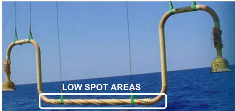
Figure 3.1: Jumper geometry with its low spot areas
