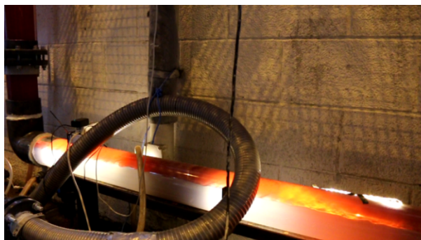
Figure 5.12: Pictures of experiment and LedaFlow model for oil displacing water at different times, 4.859 \text{ m}^3/\text{h}
