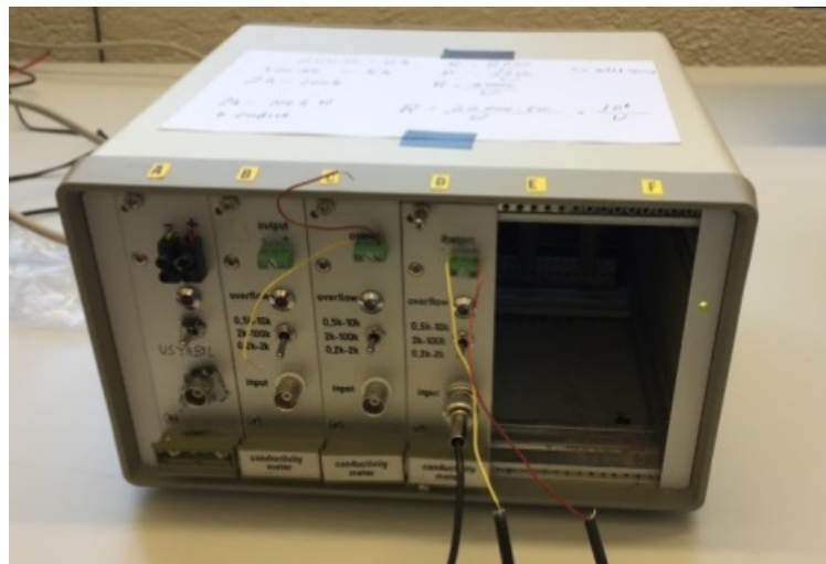
Figure 5.6: Meter 3 for measuring volume fraction
