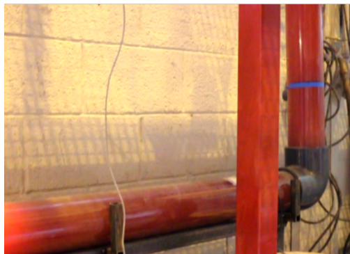
Figure F.4: Pictures of experiment and LedaFlow model at different times, for oil displacing water at 37.743 m 3 /h
