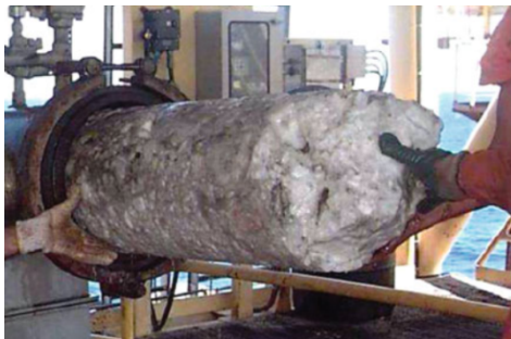
Figure 3.2: Left: Hydrate plug forming inside a pipeline, Right: Hydrate structure
