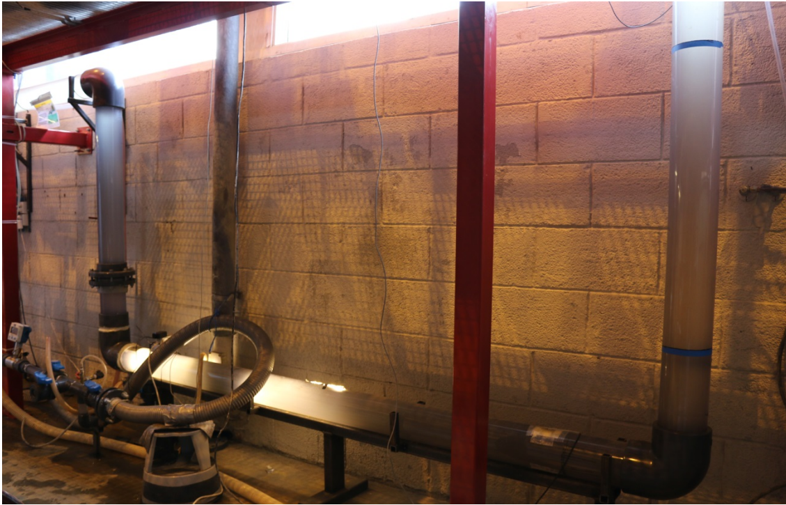
Figure 4.8: The U-jumper used for experiments
