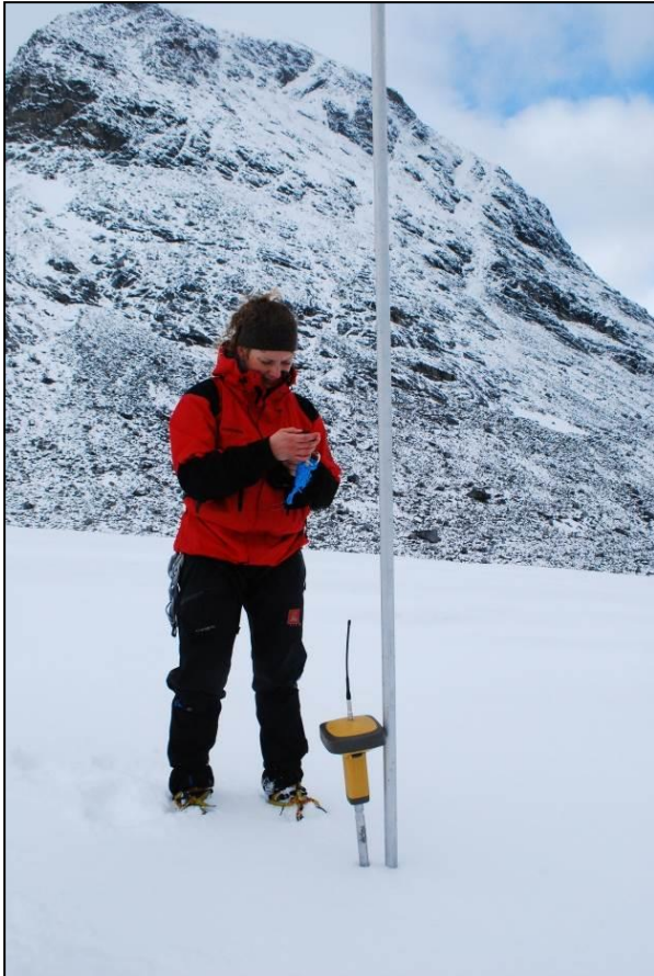
Figure 5.2. Recording handheld GPS data while the Rover is positioned as close to the stake as possible (Image: personal collection, May 2 nd 2012).
