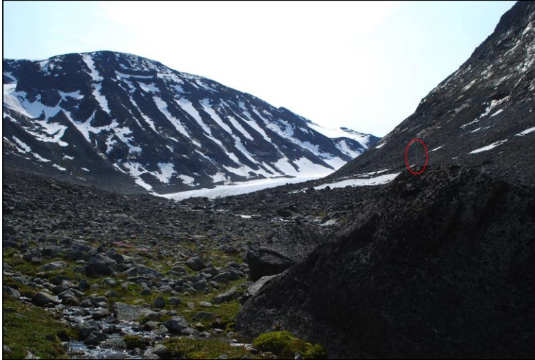
Figure 5.4. The boulder used to position the dGPS base station. Red circle indicates the threaded metal rod fixed into the rock used to screw the base in place. Hellstugubreen can be seen in the background (Image: personal collection, July 8 th 2013).
