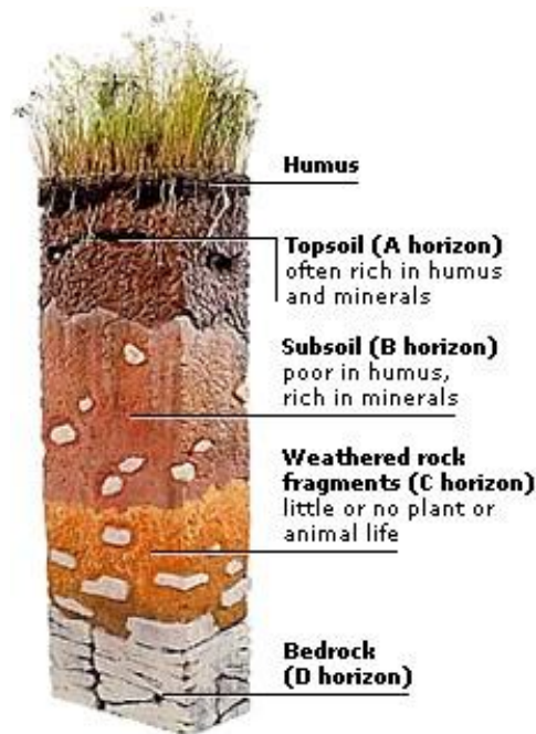
Figure 5: Soil profile horizons, horizon D demonstrates bedrock layer, horizon C presents weathered bedrock (saprolite), figure from (metropolis 2013)
