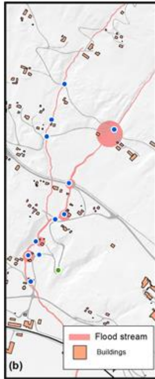
Figure 19: In the study area Brandrudsåa more than 80 % of the damage points are located in naturally flow paths. The red area marks an area of particular large erosions.
