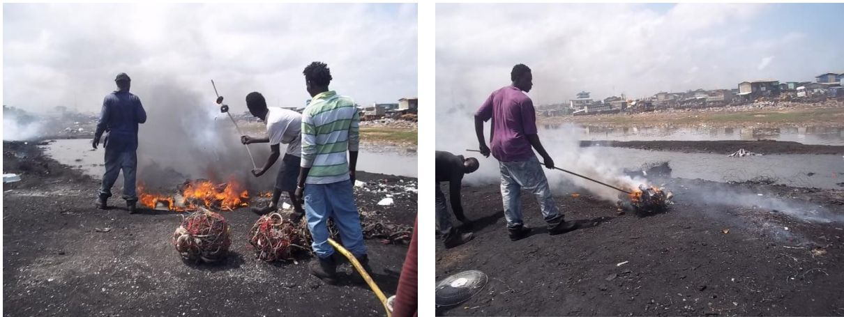
Figure 8: Burners burning the dismantled cables at the scrap yard
