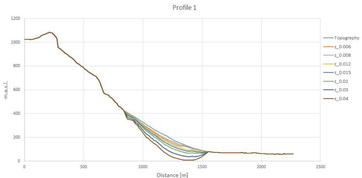
Figure 5.3: Profile lines showing computation of curvature for Profile 1. The upper, blue line represents the topography. The most suitable and realistic curvature was chosen, in this case \Delta z = 0.012 (yellow line). The same procedure is repeated for all six profile lines, results are given in (Table 6.1). All values tested are included in the figure, meaning that profile lines that are too deep or too shallow are drawn. It is not realistic with a curvature providing profiles deeper than the valley floor.
