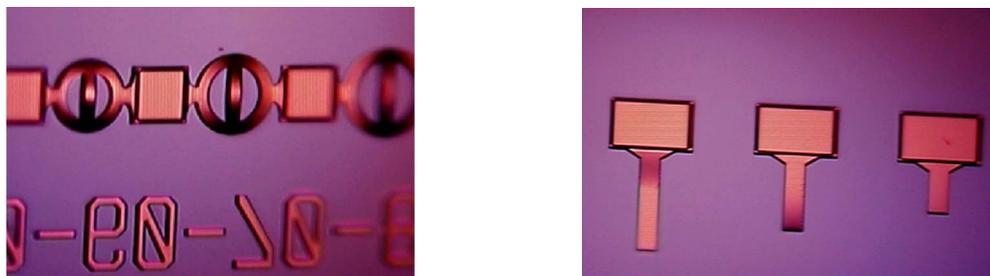
Figure 2: Optical images of buckled guckel ring and cantilever sputtered at 10 mTorr and 500 watt
