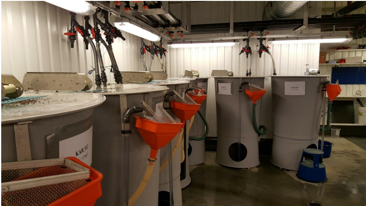
Figure 14: Picture of six of the tanks at Nofima, Sunndalsøra. The rest of the tanks are behind or beside the picture. Two plastic pipes with water goes into the tanks. These contain water from holding tanks 601 and 602 (Bye, 2017).
